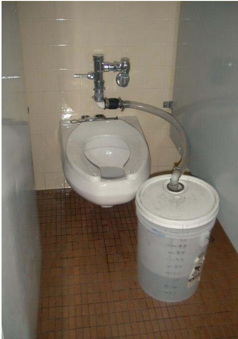
Flush Diversion Hose and Graduated Bucket
