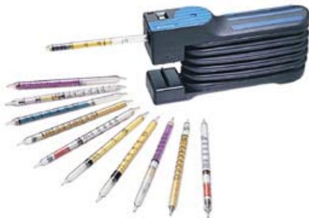
Figure 1. Dräger bellows sampler pump with tubes.
