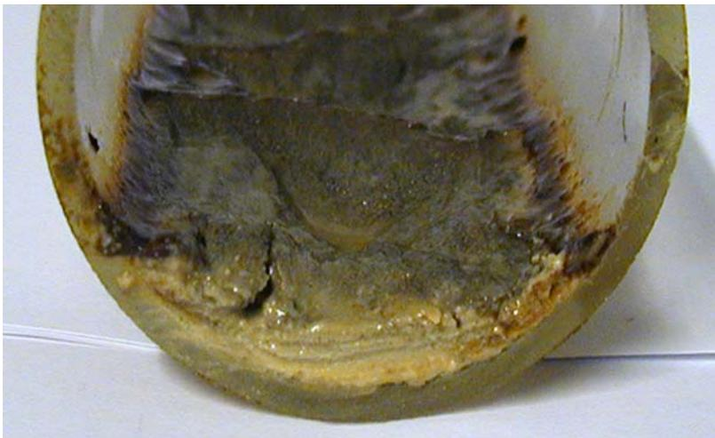
Figur 7: Build-up in the collecting drainline after nine month of use
