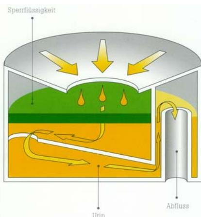
**Figur 1:** Trap with a floating sealing liquid (Source: Sinaqua-Waterless)
