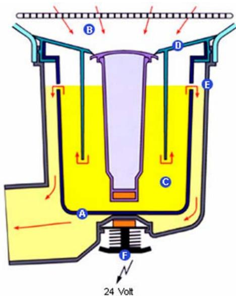
Figur 2: Trap with a buoyancy body (Source: Urimat)
