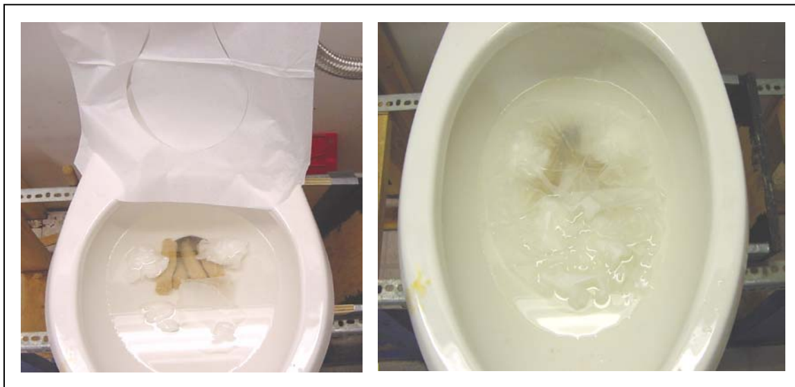
Figure 2: soybean paste and toilet paper in bowl (L), with paper seat cover added (R).
